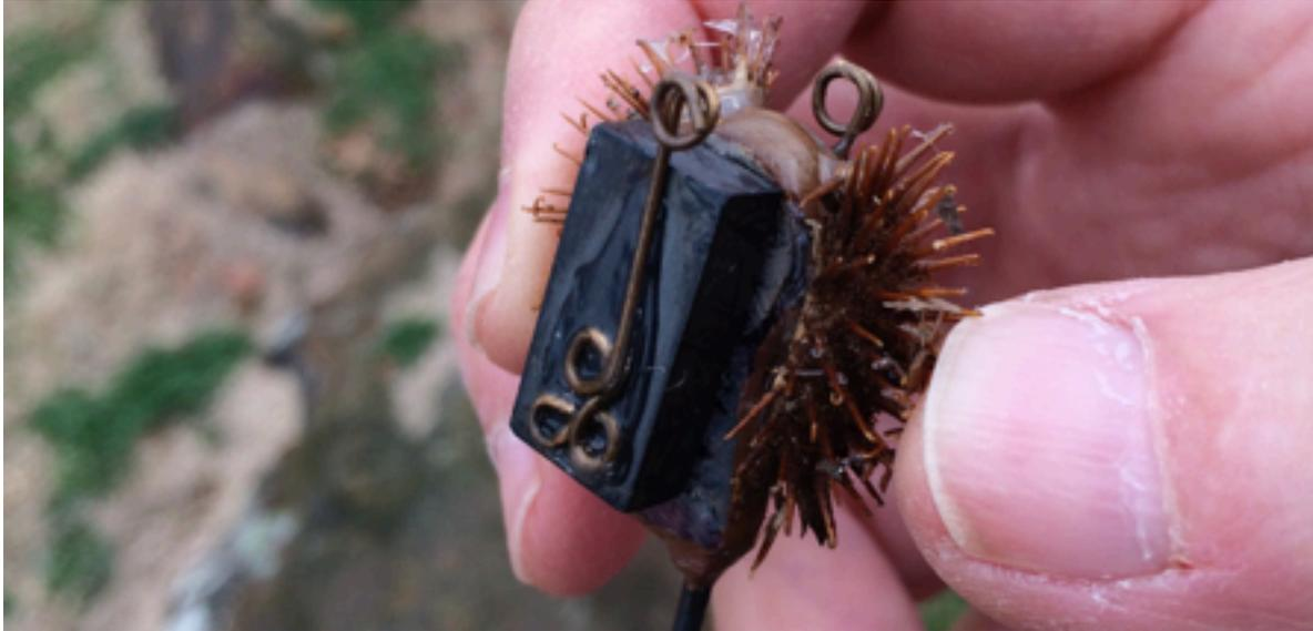
Figure 3. A close view of an NAWAC radio tag/cocklebur device. The black rectangle is the magnet. The transmitter activates when the magnet detaches.
