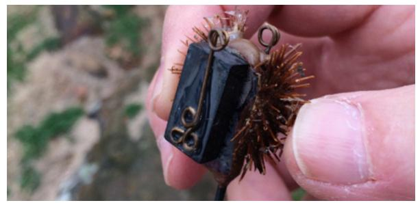
Figure 3. A close view of an NAWAC radio tag/cocklebur device. The black rectangle is the magnet. The transmitter activates when the magnet detaches.
