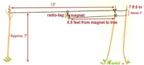
Figure 5. Original string trap set-up for radio tag 7, looking south.
