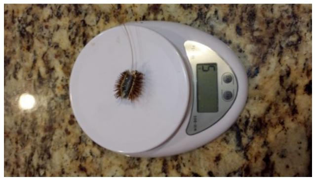
Figure 15. Dummy tag with cocklebur fruits attached
